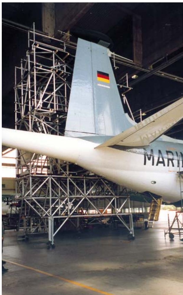
TAIL DOCK CONSISTING OF TWO HALVES MADE OF ALUMINIUM
